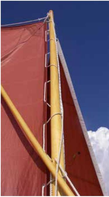
Note Spread and lacing along mast
