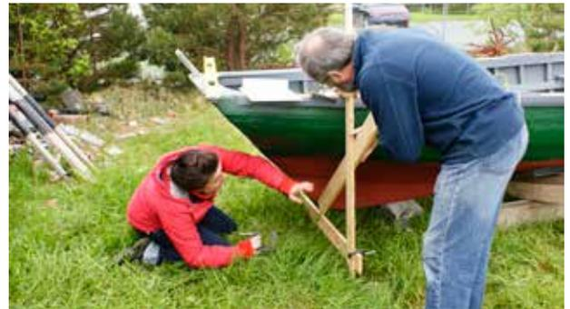
Lifting lines from Allen Brothers boat in Coley's Point
